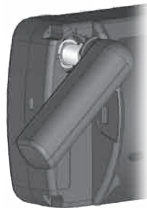
Removing the GPS Antenna
